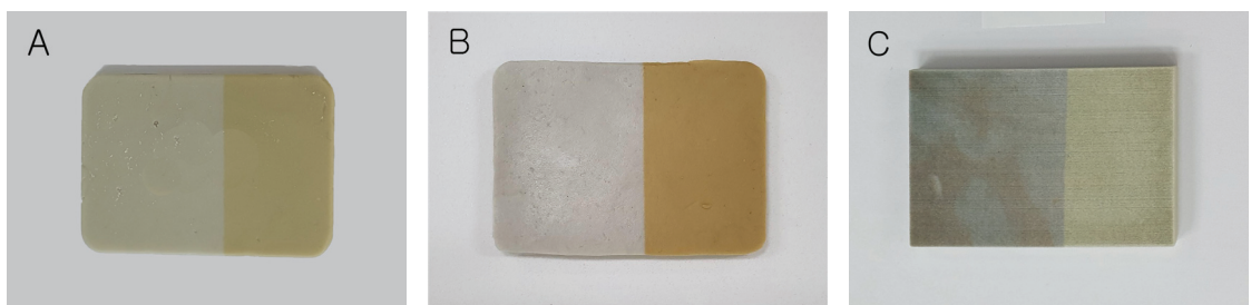
Figure 5. UV deterioration irradiation (A) AW106 + HV953U, (B) L-30, (C) CJP printout.
