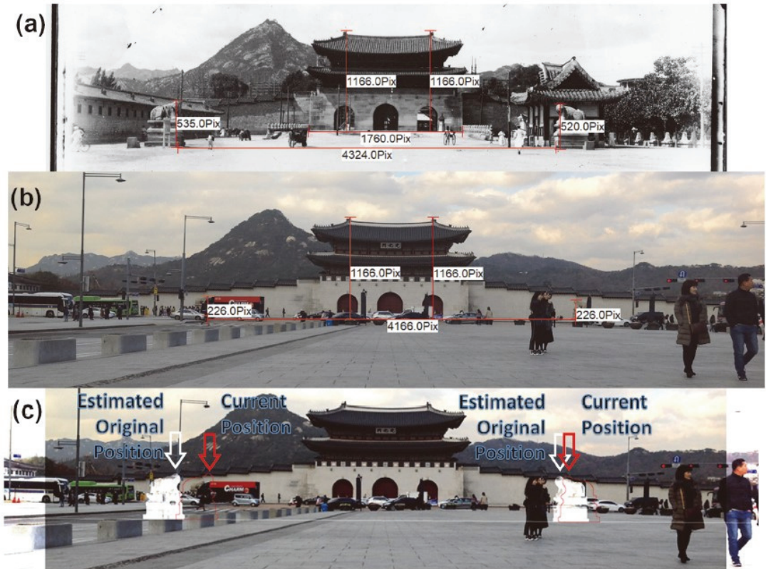
Figure 9. (a) A photograph showing both Haechi (Stone Lion) statues in the archival photo (top), (b) a recently taken photo, and (c) the extracted Haechi images from the archival photo superimposed on the recently taken photo by aligning with the skyline (Gwanghwamun Gate and Mountains on the background).
