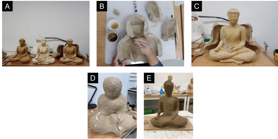
Figure 2. Production of outer mould and inner mould. (A) 3D print Iron Seated Buddha and original form of Iron Seated Buddha, (B) Engraving inside the outer mould, (C, D) Making a outer mould, (E) Making a inner mould.
